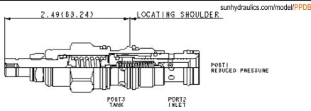
Pilot-operated, pressure reducing/relieving valves reduce a high primary pressure at the inlet (port 2) to a constant reduced pressure at port 1, with a full-flow relief function from port 1 to tank (port 3).
